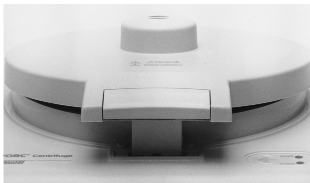
Figure 4-2. Spring-Loaded Lid Latch Mechanism
