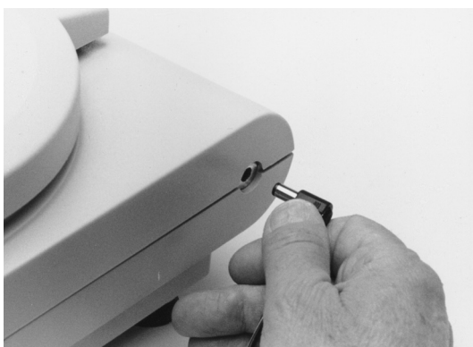
Figure 3-2. Connecting Output Cord of Power Unit to Centrifuge Jack.
