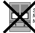
Switch 1 set for **no** internal termination
